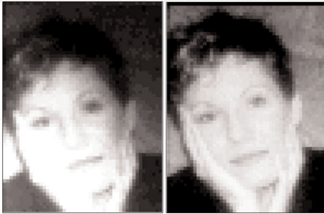
Figure 5. High frame rates aren't the only advantage of applying massively parallel processing to digital imaging. The array processors can adjust the intensity of individual pixels, improving the photographic quality of the image. Many other effects are possible by applying intelligent image-processing algorithms. (Source: Euteucus)
