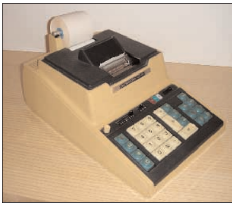
Figure 6. This is the desktop calculator that Basicom built with the Intel 4004 microprocessor and the other 4000-family chips. Federico Faggin has donated an original prototype to the Computer History Museum. (Photo: Intel.)
