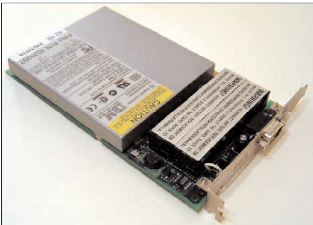
Figure 1. IBM's new SecureBlue technology adapts the security features of this IBM 4758 PCI card into licensable IP for SoCs. The PCI card is sealed inside a tamper-resistant metal enclosure. (Photo: IBM)
