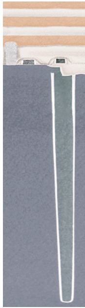
Figure 2. Conventional embedded DRAM (eDRAM) requires a deep-trench capacitor structure in addition to the transistor for each bit-cell. The capacitor trench makes the bit-cell much taller than its width and poses a problem for advanced fabrication processes.
