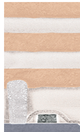
Figure 5. Z-RAM requires only one transistor, like conventional DRAM, but it doesn't need the deep-trench capacitor shown in Figure 2. As a result, it's compatible with SOI—indeed, it relies on the SOI floating-body effect to work—and it scales more easily to smaller fabrication processes.
