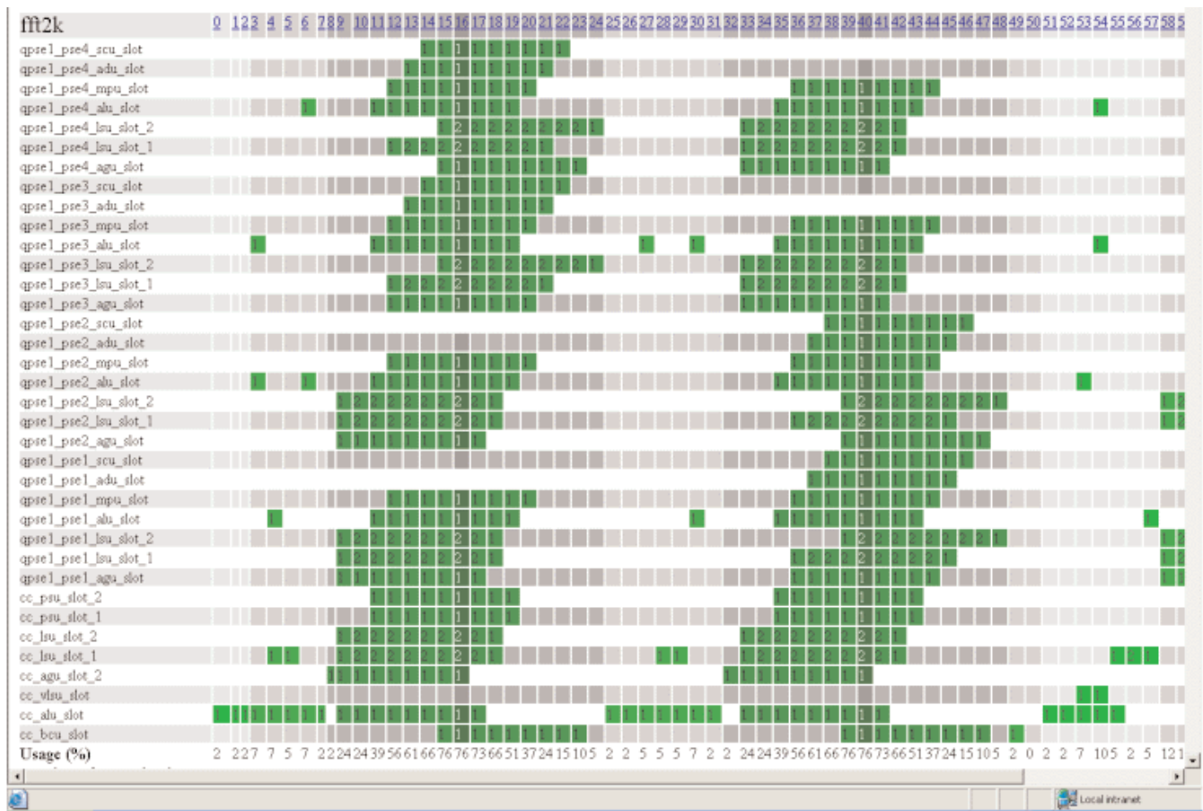
Figure 2. This screen shot of a Silicon Hive profiling tool shows an FFT executing on an Avispa ULIW core that has four PSEs and 41 instruction-issue slots. While executing the body of the innermost loop, the core keeps 31 out of 41 issue slots active (76%). Overall, the core is spending 98% of its execution time in the single-instruction, single-cycle loops of pure dataflow mode, as indicated by the darkest column of squares.
